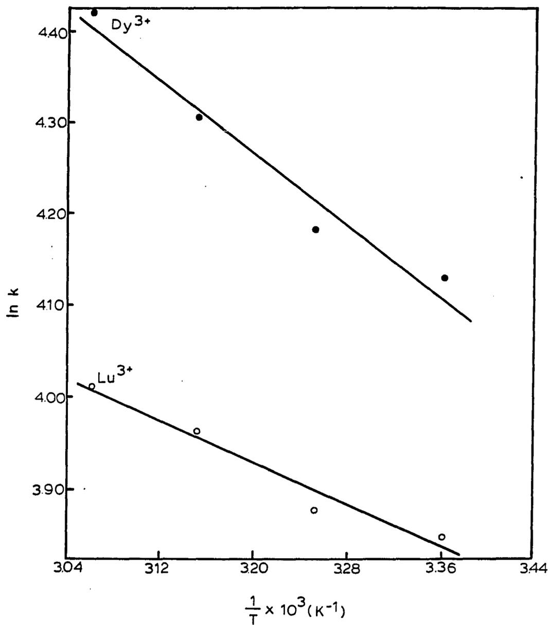
Figure 4. Plot of natural log of capacity factors of rare earth metal ions as a function of reciprocal system temperature.
