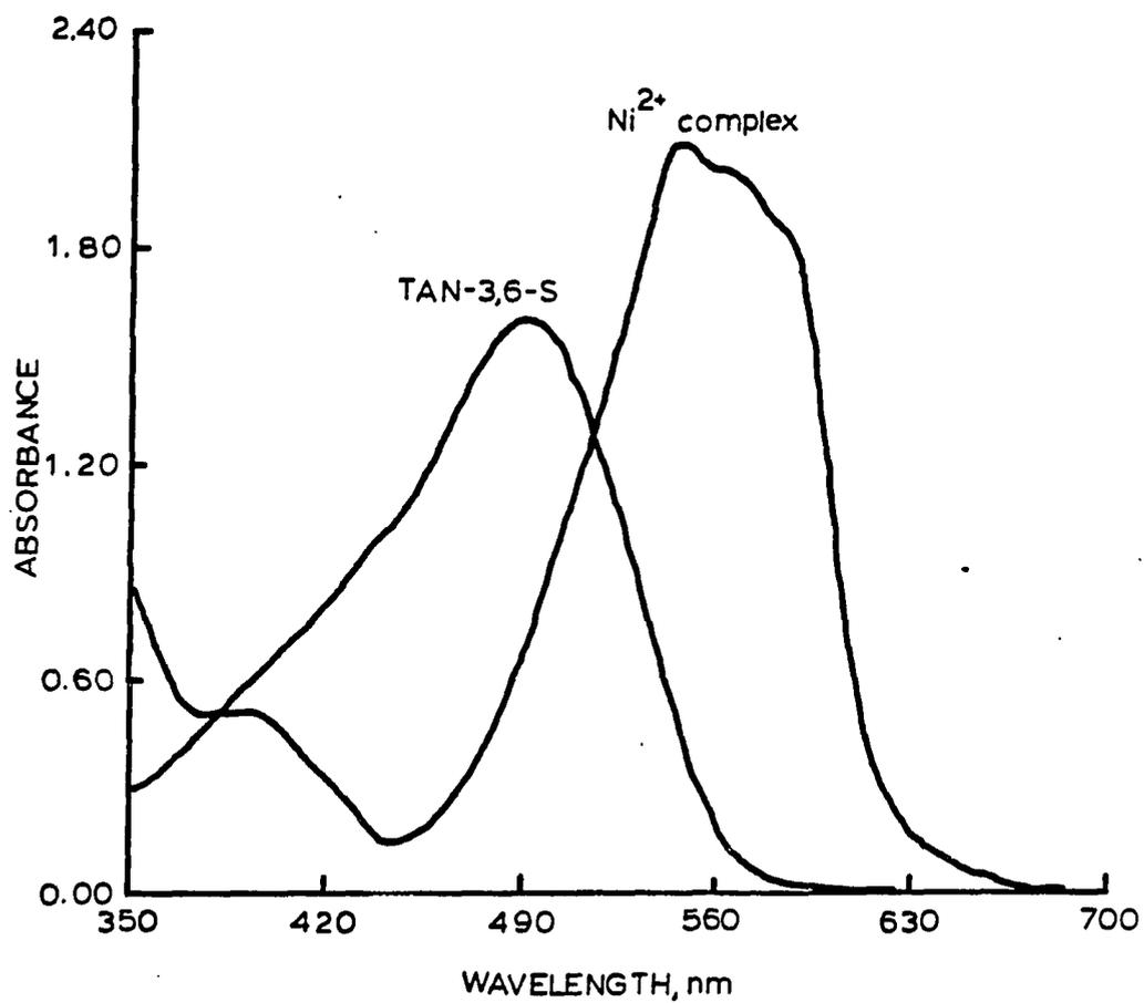
Figure 6. Visible spectra of aqueous 0.12 mM TAN-3,6-S, pH 6.2, and 0.12 mM TAN-3,6-S mixed with aqueous 0.20 mM Ni(II), pH 5.3
