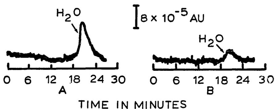
Figure 11. Chromatograms of samples containing A.) 12% water and B.) 2% water. Column was 8 mm x 10 cm TSK-SCX, eluent was acetonitrile, PCR was ET-30 in acetonitrile (0.013 g/L), eluent and PCR stream flow rates were 2.25 mL/minute, detection wavelength was 490 nm
