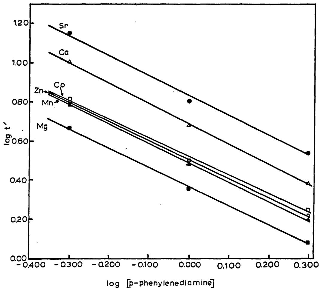
Figure 2. Plot of log adjusted retention time of divalent metal ions vs. log concentration of p-phenylenediamine. Conditions: concentrations of p-phenylenediamine used were 0.50, 1.00, and 1.99 mM, pH 3.0; temperature, 27°C; retention times normalized to correspond to a flow rate of 1.00 mL/min (actual flow rates were between 1.00 and 1.03 mL/min)
