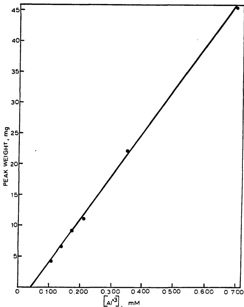
Figure 4. Calibration plot for aluminum standard solutions -- peak weight in mg vs. concentration of Al(III) in mM. Conditions: eluent, 8.23 mM p-phenylenediamine, pH 3.0; temperature, 27°C; flow rate, 0.97 mL/min. Correlation coefficient is 0.9996
