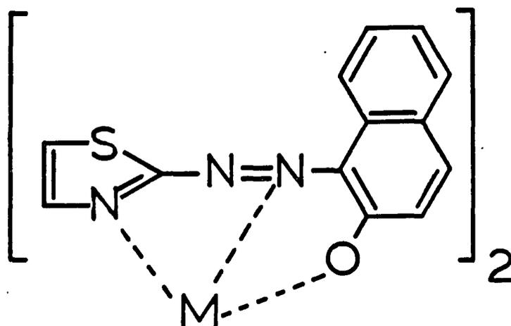
Figure 5. Structure of metal chelates which form with unsulfonated TAN (20). M = Cu(II), Ni(II), Co(II), Zn(II)
