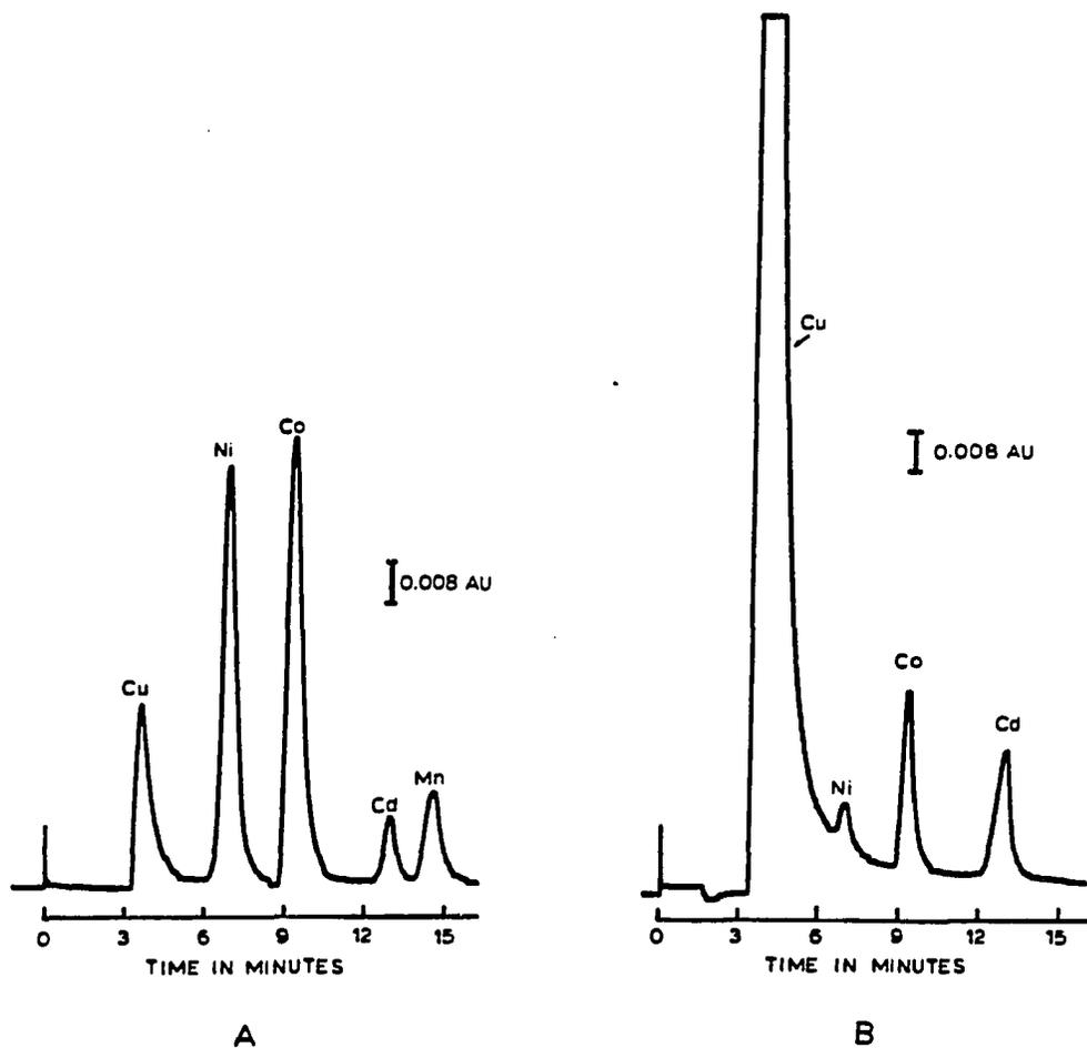
Figure 7. Separation of some transition metals on a TSKgel IC-Cation-SW silica cation-exchange column. Eluent is 3.2 mM ethylenediamine/4.0 mM tartaric acid, pH 4.5, flow rate of 0.7 mL/min. Postcolumn reagent stream is 0.09 mM TAN-3,6-S buffered with TEA, flow rate of 0.65 mL/min. Detection wavelength is 580 nm. Sample: mixture of 3.1 mM Cu(II), 0.31 mM Ni(II), 0.32 mM Co(II), 3.4 mM Cd(II), and 3.2 mM Mn(II). A.) Effluent pH = 6.9, B.) effluent pH = 4.9
