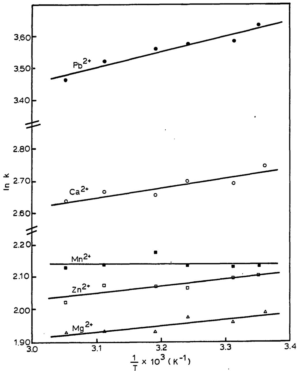
Figure 2. Plot of natural log of capacity factors of divalent metal ions as a function of reciprocal system temperature. Eluent: 0.12 M  $\text{HClO}_4$
