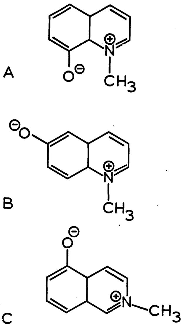
Figure 3. Structure of betaine dyes used for the spectrophotometric determination of water. A.) 1-methyl-8-hydroxyquinolinium betaine (1,8-Q), B.) 1-methyl-6-hydroxyquinolinium betaine (1,6-Q), C.) 2-methyl-5-hydroxyisoquinolinium betaine (2,5-IQ)
