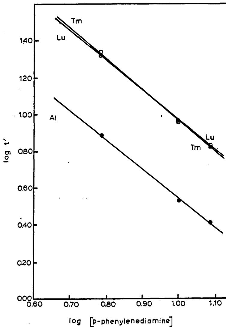
Figure 3. Plot of log adjusted retention time of trivalent metal ions vs. log concentration of p-phenylenediamine. Conditions: concentrations of p-phenylenediamine used were 6.04, 9.91, and 12.07 mM, pH 3.0; temperature, 27°C; retention times normalized to correspond to a flow rate of 1.0 mL/min (actual flow rates were between 0.96 and 1.0 mL/min)
