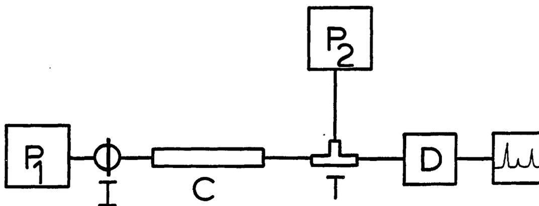
Figure 1. A typical postcolumn reaction chromatographic system. P<sub>1</sub> = eluent pump, I = injection valve, C = separation column, T = mixing or reaction chamber, P<sub>2</sub> = reagent pump, D = detector
