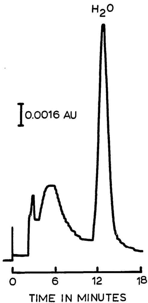
Figure 16. 0.138% water in a methanolic solution of 1.15 M 3-mercaptopropionic acid. Sample loop: 20 microliters. Separation column: 8 mm x 10 cm. Flow rate: 1 mL/min. Other conditions given in text
