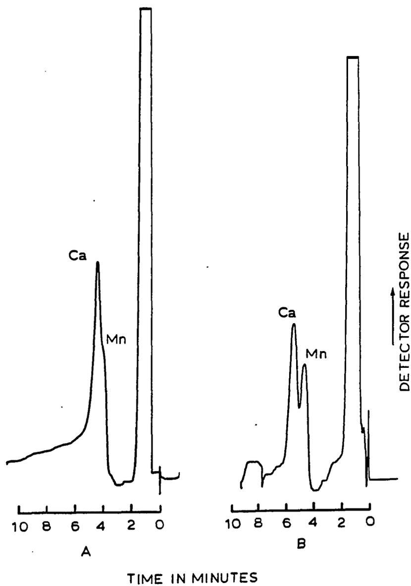
Figure 6. Separation of  $Mn^{2+}$  and  $Ca^{2+}$ . Eluent: 1.0 mM ethylenediamine, 2.0 mM tartaric acid, pH 4.5. A.) Temperature: 25°C, B.) Temperature: 54°C
