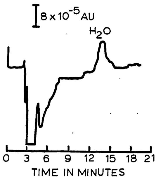
Figure 19. Limit of detection as obtained with the long separation column (8 mm x 10 cm): 260 ng water. Injected: 12.8 ppm water in methanol. Sample loop: 20 microliters. Flow rate: 1 mL/min. Other conditions given in text
