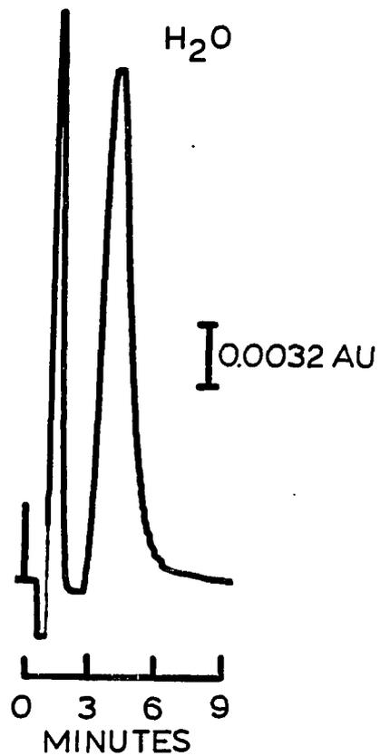
Figure 17. 367 ppm water in isopropanol. Sample loop: 100 microliters. Separation column: 4.6 mm x 5 cm. Flow rate: 0.8 mL/min. Other conditions given in text
