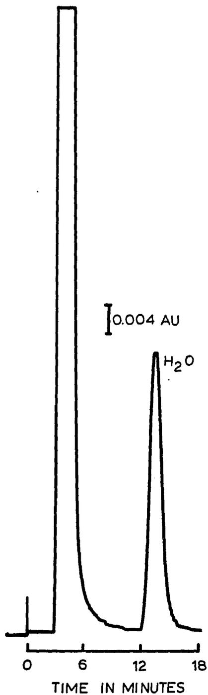
Figure 15. 0.321% water in acetone. Sample loop: 20 microliters.
