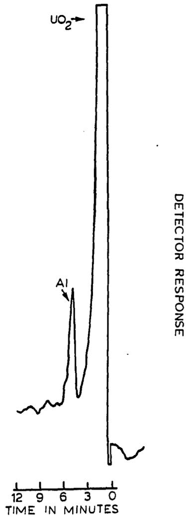
Figure 6. Separation of Al(III) from  $\text{UO}_2^{2+}$ . Concentration of Al(III) is 0.173 mM, concentration of uranyl ion is 19.80 mM. Conditions as in Figure 4
