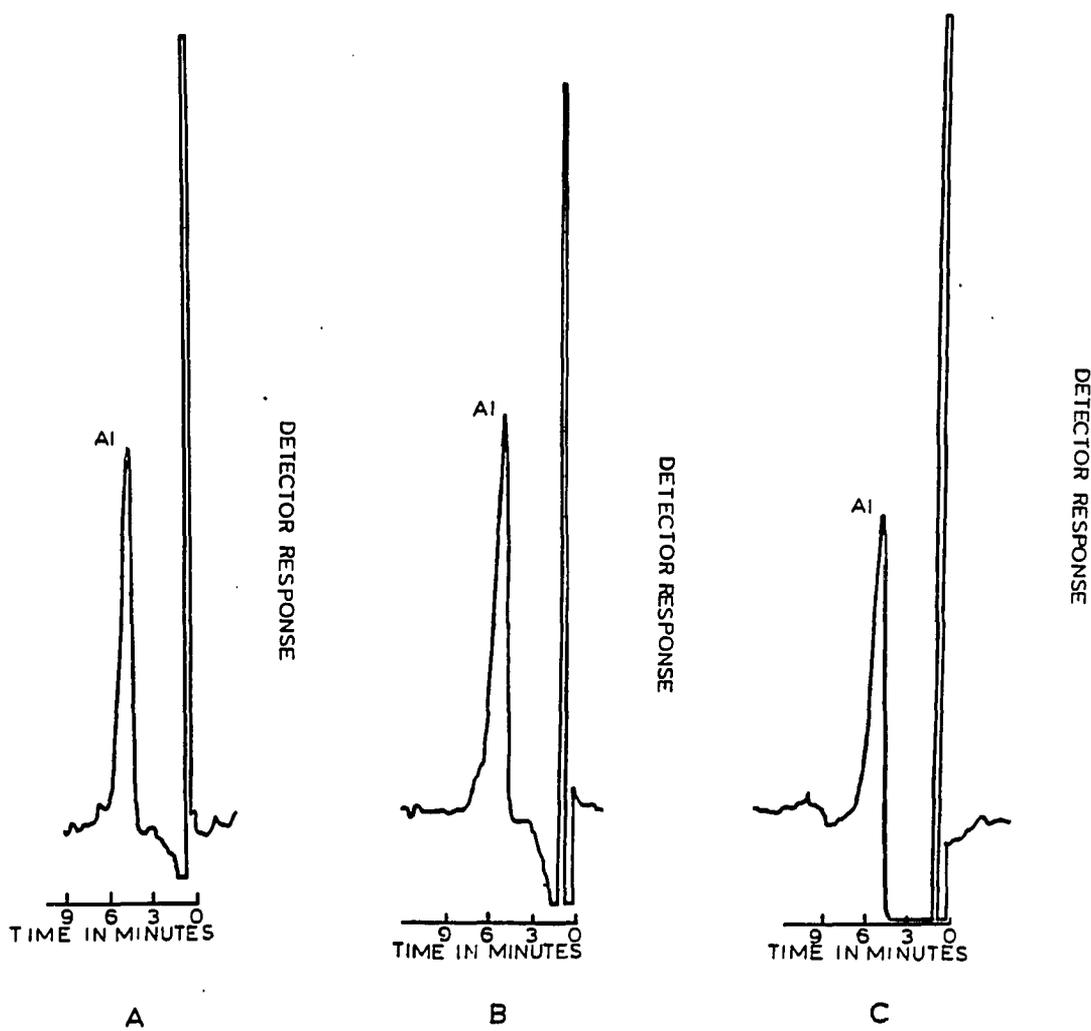
Figure 5. Conditions as in Figure 4. A.) Standard 0.349 mM Al(III) solution, B.) solution of NBS Standard Sample 94a, 0.383 mM in Al(III), pH 2.94, C.) solution of NBS Standard Sample 94a, 0.383 mM in Al(III), pH 0.95
