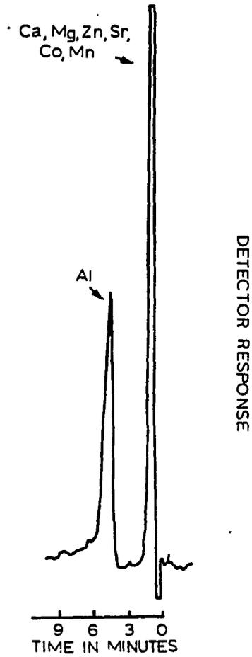
Figure 7. Separation of Al(III), 0.286 mM, from six other metal ions: 3.44 mM Ca(II); 3.77 mM each of Mg(II), Zn(II), Sr(II); 4.10 mM each of Co(II), Mn(II). Conditions as in Figure 4
