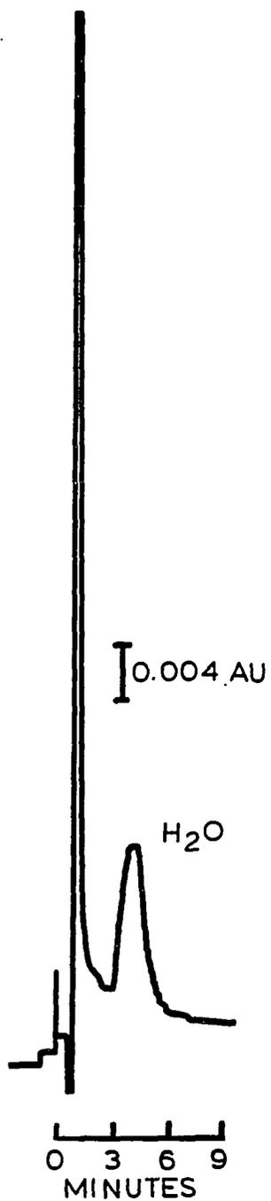
Figure 18. 184 ppm water in toluene. Sample loop: 100 microliters.
