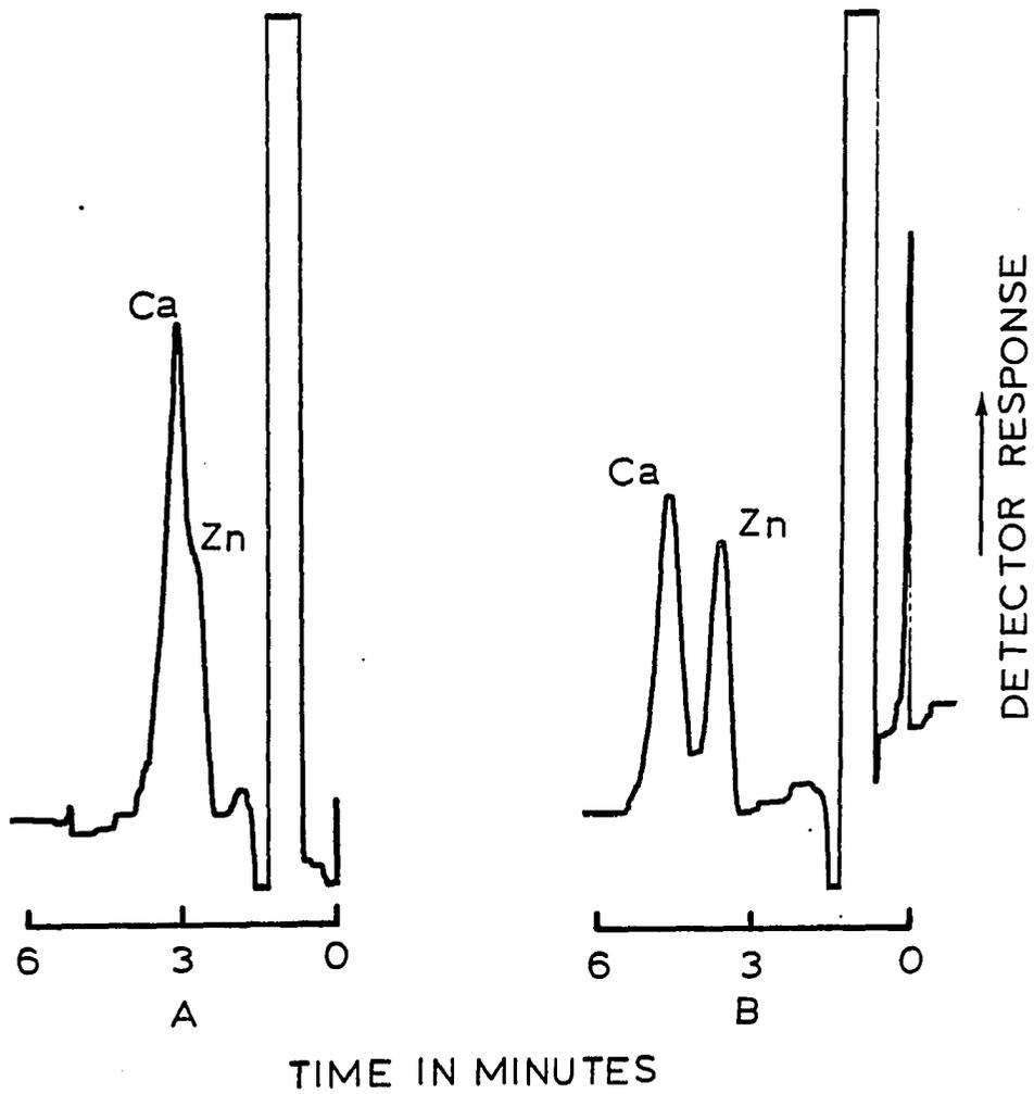
Figure 7. Separation of  $Zn^{2+}$  and  $Ca^{2+}$ . Eluent: 3.0 mM p-phenylenediamine dihydrochloride. A.) Temperature: 27°C, B.) Temperature: 57°C
