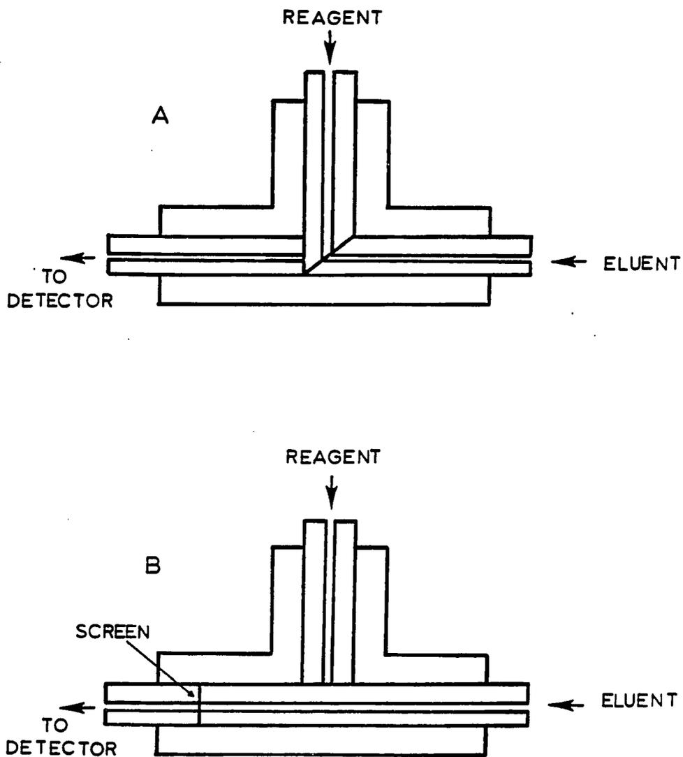
Figure 2. Mixing tees used for combining effluent and reagent streams in a postcolumn reaction chromatographic system. A.) Design by Elchuk and Cassidy (3), B.) design by Cassidy et al. (2)
