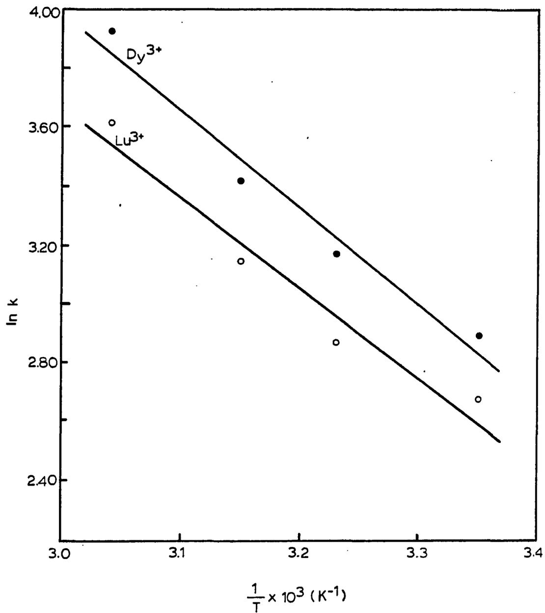
Figure 5. Plot of natural log of capacity factors of rare earth metal ions as a function of reciprocal system temperature. Eluent: 7.8 mM p-phenylenediamine dihydrochloride
