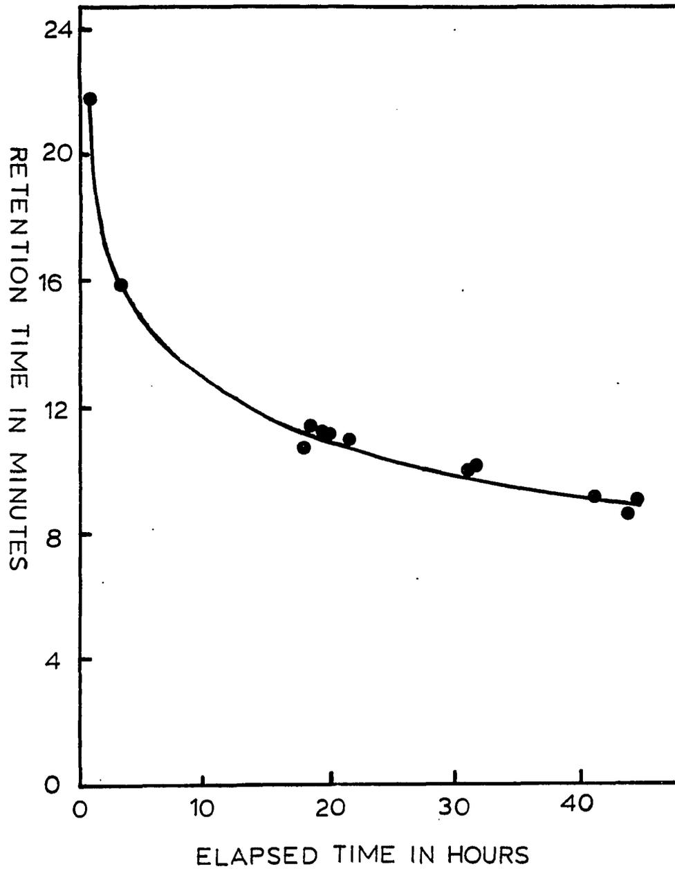
Figure 1. Plot of the retention time of Al(III) peak vs. time elapsed since column equilibration achieved. Conditions: eluent, 0.994 mM N-phenylethylenediamine, pH 3.1; temperature, 26°C; flow rate, 1.02 mL/min
