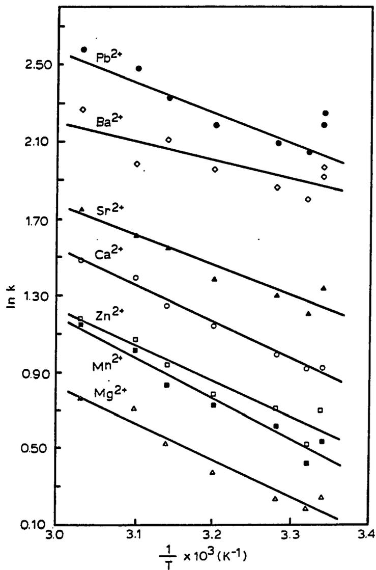
Figure 3. Plot of natural log of capacity factors of divalent metal ions as a function of reciprocal system temperature. Eluent: 3.0 mM p-phenylenediamine dihydrochloride
